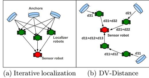
Figure 4: Distributed localization techniques - iterative localization and DV-Distance - can localize a sensor robot in the remote regions of a tank.
