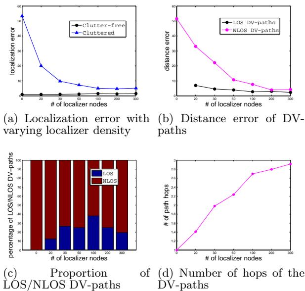
**Figure 7: Effect of localizer density on the localization accuracy of DV-Distance in cluttered environments. Each data point is an average of 100 sample runs.**
