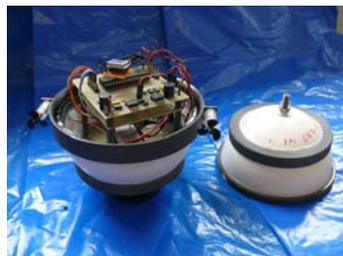
(c) Submersible underwater robot prototype (Courtesy: Simon Watson, University of Manchester)
