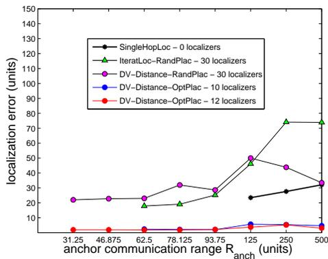
**Figure 10: Comparison between the error of localization techniques using random localizer placement and optimal localizer placement. Each data point is an average of 50 simulation runs.**
