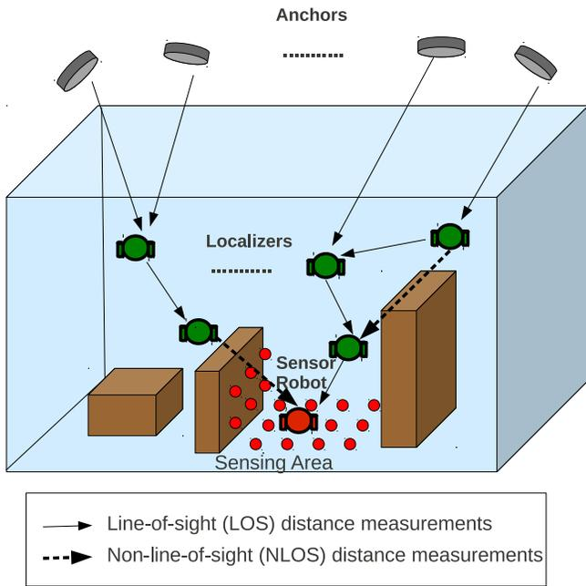
(a) Localization of the sensor robot in the (discretized) sensing area. Anchors, at the surface, and deployed localizer robots enable the localization of the sensor robot. The cluttered environment gives rise to NLOS measurements.
