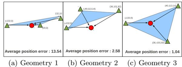
**Figure 2: Effect of reference geometry on localization error.** The line-of-sight (LOS) measurements are contaminated with Gaussian noise  $\mathcal{N}(0,1)$ . The position error is an average over 10000 samples.
