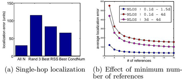
Figure 3: Localization error in single-hop localization with NLOS distance measurements. Each data point is an average of 10000 samples.
