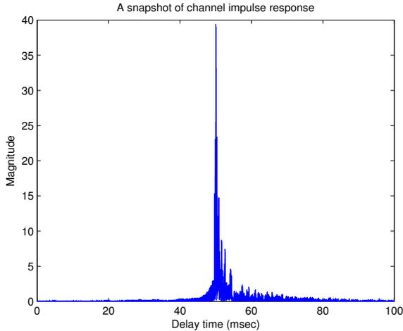
**Figure 1: A snapshot of the channel impulse response at the first receiving hydrophone, obtained by using the LFM signal.**
